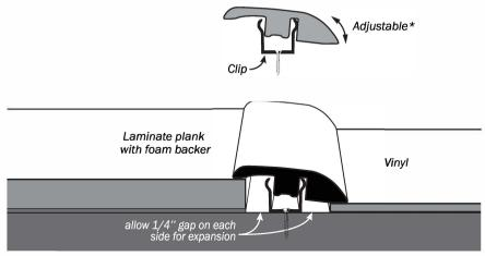
\* Adjust the position of the molding in the clip based on the height of the lower surface flooring
